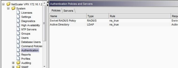
The authentication must be then added such as the Access Gateway/Virtual Servers menu. If just Swivel authentication is required then ensure that only the Swivel policy is active for the Primary. If you require AD and Swivel authentication then you need to make active the Swivel policy as the secondary. Save the settings.
