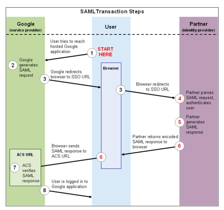
The Identity Provider (IdP) authenticates the user. If the authentication is successful it creates a SAML response and posts that response to the url of the Google Apps ACS that it was passed in the SAML request. The ACS then allows the user access as appropriate.
