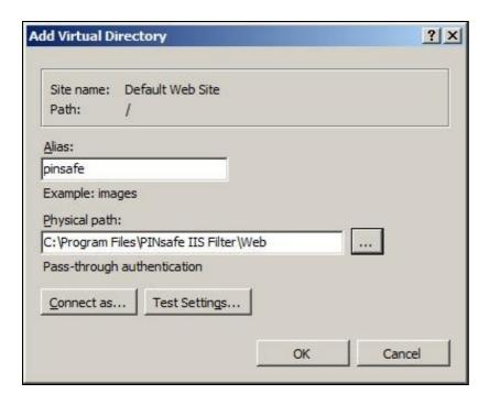
3. Point the path to the PINsafe directory Web folder, by default C:\Program Files\PINsafe IIS Filter\Web. Test Connection verifies the path, and Connect As allows Application User for pass through authentication.
