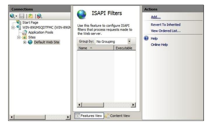
4. Select the Path to the Swivel ISAPI filter. Note that the actual file you require will be PINsafeIISFilter.dll, located in the sub-folder Web\bin of the installation folder. Enter a name for the Filter such as *PINsafe ISAPI Filter*. When information is complete click on Ok.
