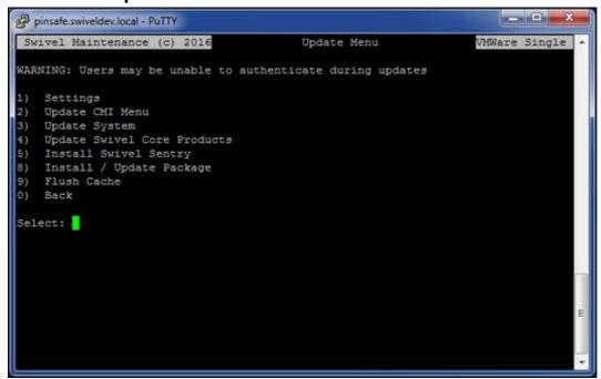
The Update Menu is located in the Console Management Interface of the Swivel Appliance. Please see the PuTTY How To Guide for guidance on connecting to the appliance via SSH. From the Main menu, select the Administration menu, then Update Appliance.
