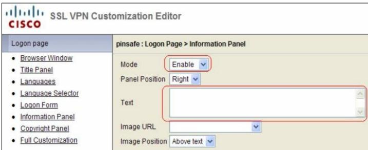
Change Mode to ?Enable?. Modify the pinsafeurl variable in the Cisco ASA 8 customisation Script to reflect your Swivel server?s URL. (The scripts are located at the top of the page under prerequisites). Paste the modified content into the Text box. Click on Save on the top right corner of the Customization Editor to save the object.
