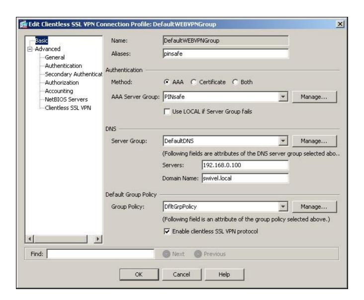
Click on Advanced then Clientless SSL VPN. Select the customization object created and add a Group URL used to access the ASA with Swivel authentication.
