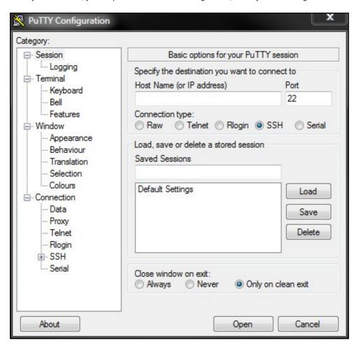
To connect to the Swivel appliance enter the IP address of the PINsafe appliance into the Host Name field (the default out of the box IP address is 192.168.0.35 for the standalone appliance).
