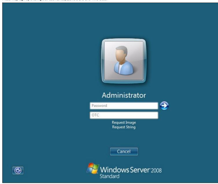
The one time code can be sent by an SMS message or a mobile phone client. Do not click Get Message unless the image is to be used for authentication.
