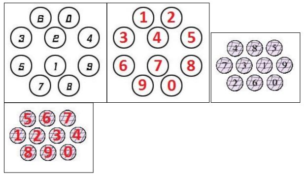
BUTton Image, the PIN is arranged as a telephone keypad, and the PIN extraction relates to the PIN numbers in the pad. The red numbers show the default PIN number settings. The One Time Code is derived from the numbers displayed in their pattern. Each image is unique and the numbers change position each time. (Note BUTton is not related to the Pinpad).
